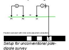
main in the deeper seam, as well as a buried highwall associated with the shallow seam. In terms of a resistivity target, the mine workings at a depth of 90 feet represent a much more complicated target than the previous two case histories, considering its depth and complex conditions above the seam, including strip mining and auger mining of a shallower seam.
