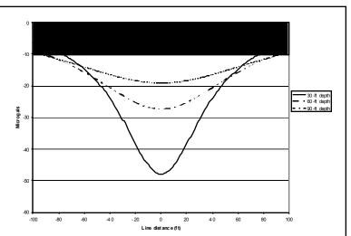
Theoretical response of the gravity method over a 20-foot diameter air-filled tunnel – a water-filled tunnel would have about a third of this response.
