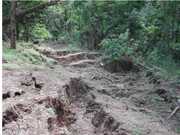
Figure 9. Surface expression of progressive failure
