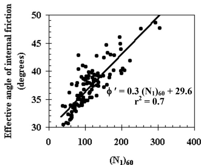
Figure 8. Correlation between angle of internal friction of CCR and normalized SPT data.
