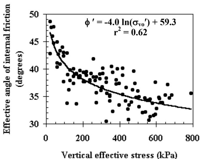
Figure 9. The angle of internal friction of coal refuse material decreases by increasing the confining effective stress.
