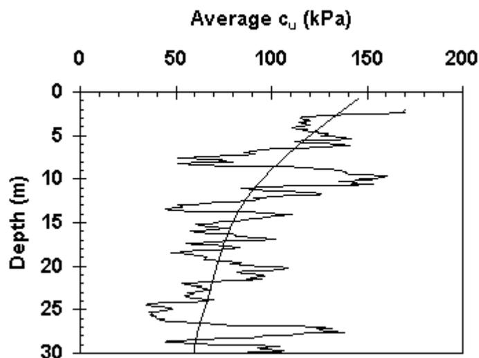
Figure 7. Average undrained shear strength of FCR with depth based on cone data at sites in western PA.
