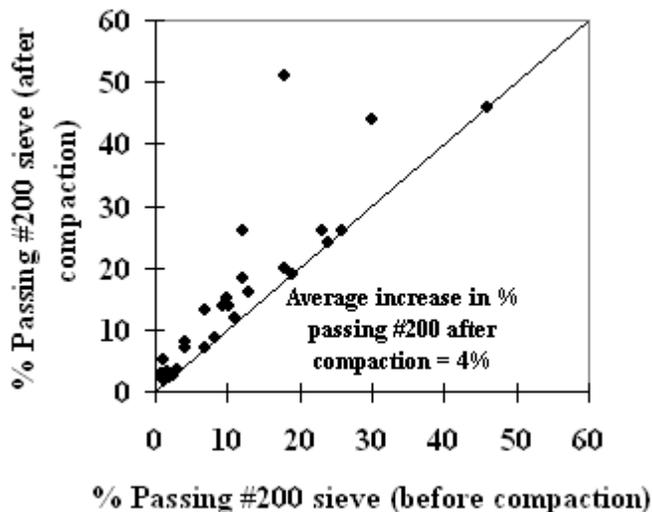
Figure 4. Effect of compaction on CCR fines content.
