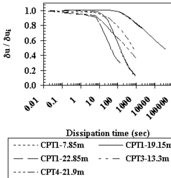
Figure 5. Piezocone dissipation tests at sites in western PA.
