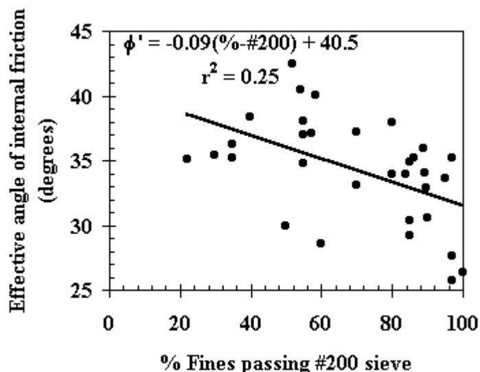
Figure 7. Effective angle of internal friction of FCR decreases with increasing % fines.
