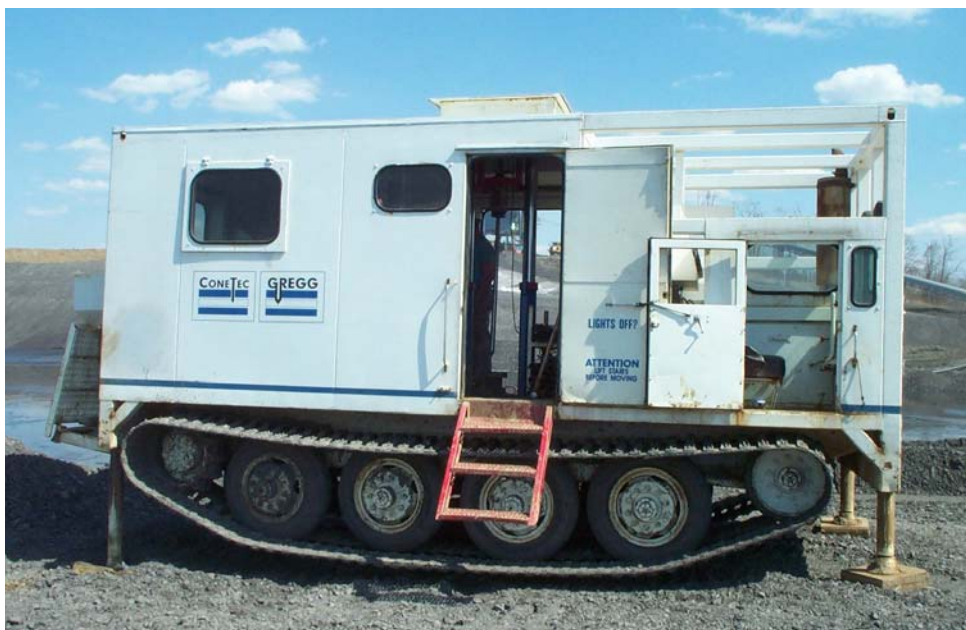
Cone penetration test rig positioned on platform during testing.
