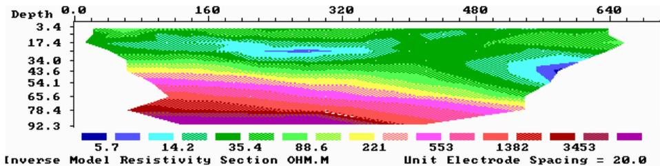
*E-W resistivity profile across fine coal refuse lagoon. The base of the coal refuse in contact with bedrock is clearly visible (approximately the yellow line), and the variations in resistivity identified from the EM-31 can be observed as a function of depth.*
