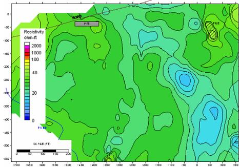
*Distribution of shallow ground resistivity from EM-31 measurements.*
