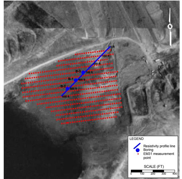
*Location of EM measurement points and resistivity profile at one of the La Belle property slurry pond.*
