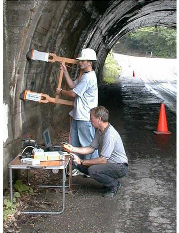
Non-destructive testing of concrete with Ground Penetrating Radar (GPR) at Rich Hill Road test site.
