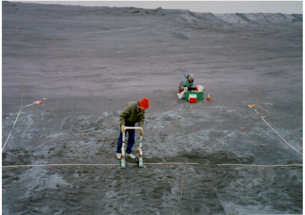
Acquisition of the 3-D GPR data set using a pulseEKKO IV Digital Recording System with 200-MHz antennas. The work was performed in an old copper mine tailings area.
