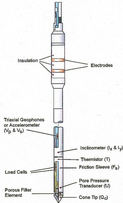
*Schematic of instrumented CPTU device.*
