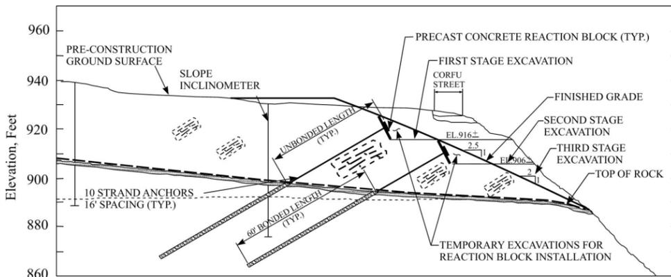
*Schematic cross section of Corfu Street slope stabilization.*
